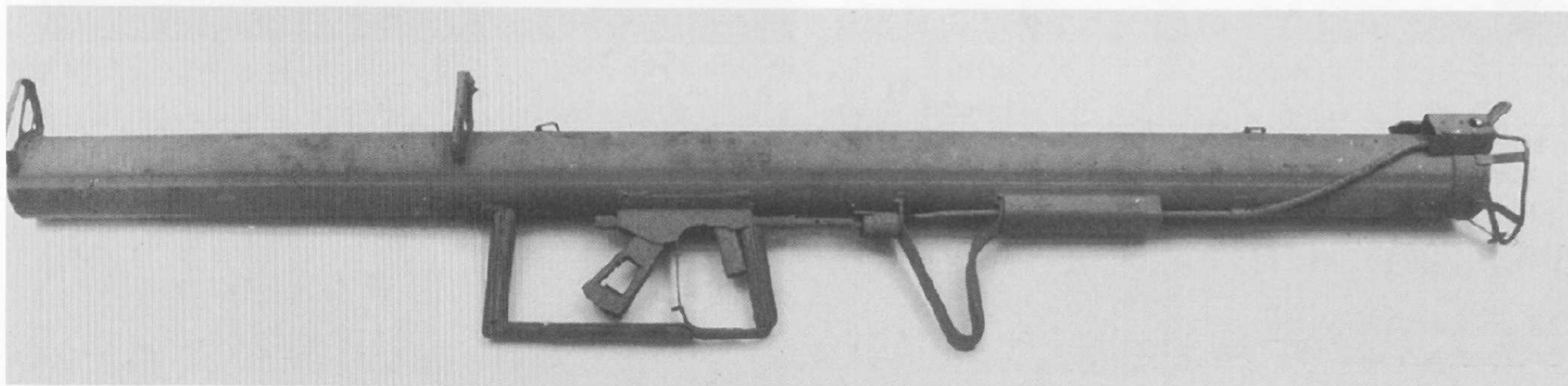
The early form of the Raketenpanzerbüchse. A protective shield with a sighting window was added only later. The equipment of a mountain Jäger division in 1944 was supposed to include 117 of them.
