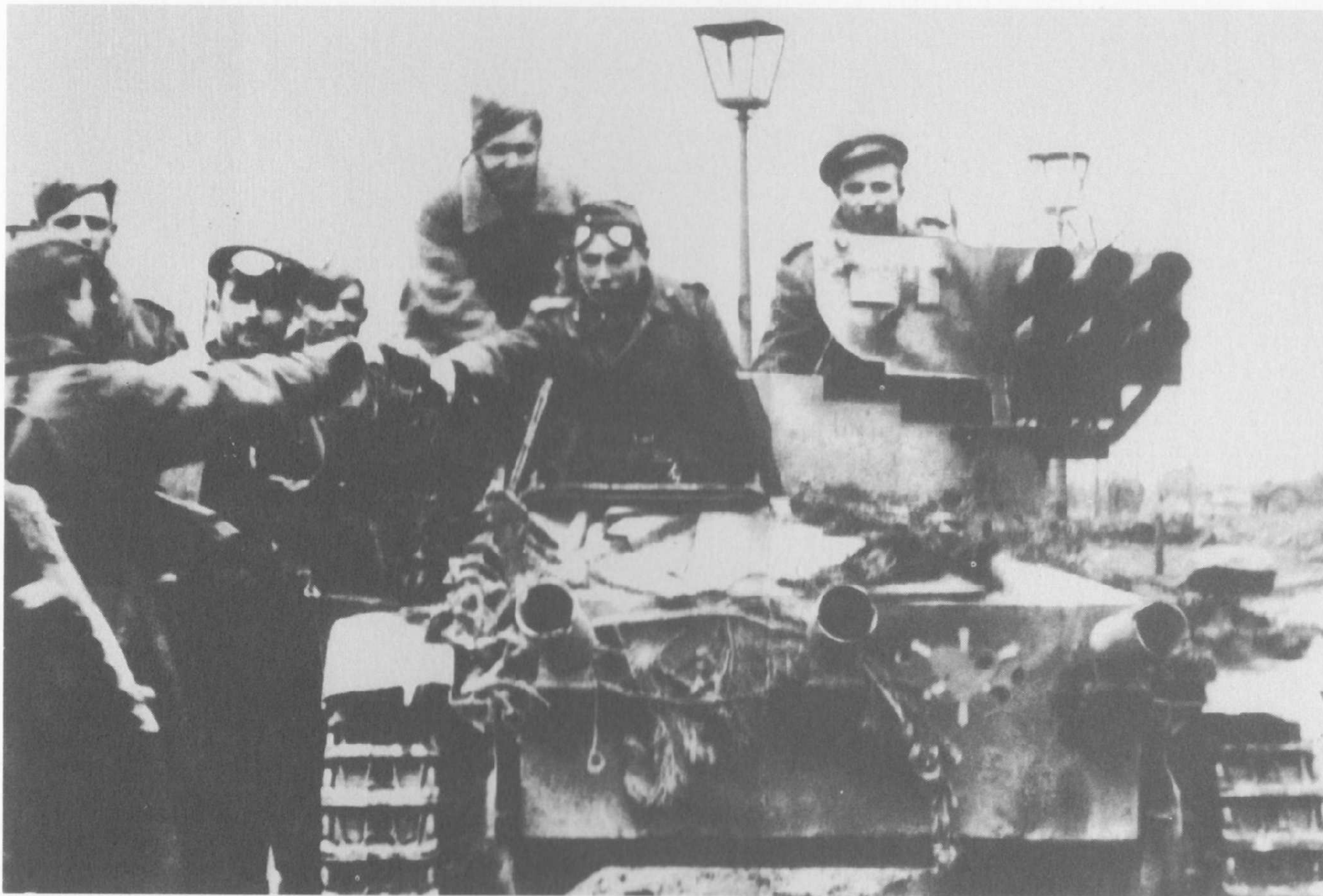
Raketenpanzerbüchse 54 (sixfold) on Heavy Load Carrier B-IV. Six "Panzerschreck" were combined to form one block, mounted with traverse on the chassis of an armored vehicle. Tanks were to be attacked at short range by the shotgun principle.
